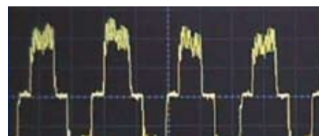
Wave generated by a traditional inverter.
